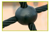
**5- The 16mm diameter ropes** are made of galvanised steel cable covered with polyester. The cables are linked together and held in place by injected polyamide spheres.
