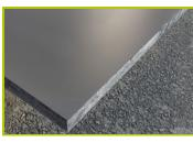
12-The blades of the gangway floor are made of polyethylene, 20mm thick.
