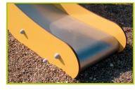
4- The sliding surfaces are made of 2mm thick stainless steel, which is shaped, bent and rolled from one piece.
