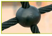
5- The 16mm diameter ropes are made of galvanised steel cable covered with polyester. The cables are linked together and held in place by injected polyamide spheres.
