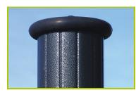
1- The 125mm diameter posts are made of painted galvanised steel, ensuring robustness and durability. The caps are made of injection moulded polyamide.
