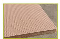
4- The seat is made from a 12.5mm thick textured and non-slip compact material (HPL).
