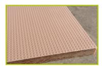
7- The climbing wall is made from a 12.5mm thick textured and non-slip compact material (HPL).
