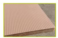
**9- The unstable platform** is made from a 12.5mm thick textured and non-slip compact material (HPL).
