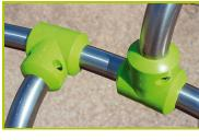
**12-Injection moulded polyamide fixings** connect the posts with the platforms and the various play features. They are non-toxic, flameproof and U.V. resistant. The thickness of the polyamide makes the equipment both strong and vandal resistant.
