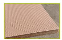
**2- The platform and the seats** are made from a 12.5mm thick textured and non-slip compact material (HPL).
