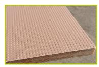
**3- The platform and the steps** are made from a 12.5mm thick textured and non-slip compact material (HPL).
