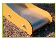
8- The sliding surface is made of 2mm thick stainless steel, which is shaped, bent and rolled from one piece.
