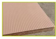
4- The platform and the steps are made from a 12.5mm thick textured and non-slip compact material (HPL).
