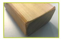
**3- The panels** are made from larch (plank sizes 45 x 68mm). Larch is naturally resistant and long lasting.
