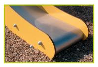
**7- The sliding surfaces** are made of 2mm thick stainless steel, which is shaped, bent and rolled from one piece.
