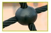
**7- The 16mm diameter ropes** are made of galvanised steel cable covered with polyester. The cables are linked together and held in place by injected polyamide spheres.
