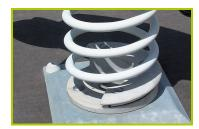
**3- The springs** are made from Grade 35SCD6 steel, shot blasted, stress relieved, zinc coated and finished with two coats of epoxy polyester powder.
