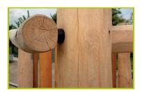
1- The posts with average diameter 120 to 140mm are made from sap free robinia. The robinia is sanded and has had its bark removed. Robinia is naturally rot proof and does not require any additional chemical protection; it is equally extremely resistant to attacks from external sources (insects, fungi, climatic variations), guaranteeing the long term durability of the playground equipment.
