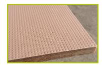
**3- The platforms** are made from a 12.5mm thick textured and non-slip compact material (HPL).
