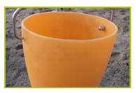
**5- The buckets** are made of rotomoulded polyethylene.
