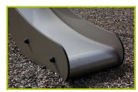
10-The sliding surface is made of 2mm thick stainless steel, which is shaped, bent and rolled from one piece. The sides are made from a 13mm thick compact material (HPL).
