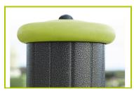
**2-** The 125mm diameter posts are made of painted galvanised steel. The two-tone grey grained finish has a slightly undulating surface for increased scratch resistance. The caps are made of injection moulded polyamide.
