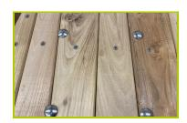
1- The boards are made from sap free robinia (plank sizes: 22 / 27mm). The robinia is sanded and has had its bark removed. Robinia is naturally rot proof and does not require any additional chemical protection; it is equally extremely resistant to attacks from external sources (insects, fungi, climatic variations), guaranteeing the long term durability of the playground equipment.
