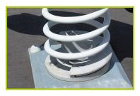
**3- The springs** are made from Grade 35SCD6 steel, shot blasted, stress relieved, zinc coated and finished with two coats of epoxy polyester powder.
