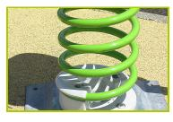
4- The spring is made from Grade 35SCD6 steel, shot blasted, stress relieved, zinc coated and finished with two coats of epoxy polyester powder.
