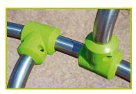
**3- Injection moulded polyamide fixings** connect the posts with the platforms and the various play features. They are non-toxic, flameproof and U.V. resistant. The thickness of the polyamide makes the equipment both strong and vandal resistant.
