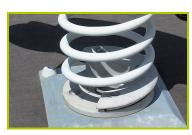
3- The springs are made from Grade 35SCD6 steel, shot blasted, stress relieved, zinc coated and finished with two coats of epoxy polyester powder.
