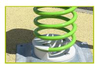
**4- The springs** are made from Grade 35SCD6 steel, shot blasted, stress relieved, zinc coated and finished with two coats of epoxy polyester powder.
