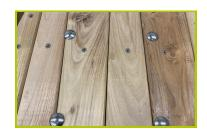
1- The boards are made from sap free robinia (plank sizes: 22 / 27mm). The robinia is sanded and has had its bark removed. Robinia is naturally rot proof and does not require any additional chemical protection; it is equally extremely resistant to attacks from external sources (insects, fungi, climatic variations), guaranteeing the long term durability of the playground equipment.
