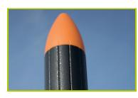
1- The 125mm diameter posts are made of painted galvanised steel. The grained finish has a slightly undulating surface for increased scratch resistance. The caps are made of rotary moulded polyethylene.
