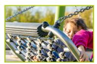
2- The braided rope seat is made of galvanised steel, covered in polyester. The connecting parts are in painted aluminium. The seat is fitted to a stainless steel frame structure, made up of two 40 mm diameter posts, and is suspended from small link stainless steel chains.
