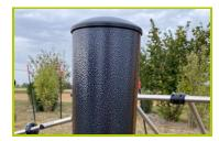
1- The 125mm diameter post is made of painted galvanised steel. The two-tone grey grained finish has a slightly undulating surface for increased scratch resistance. The cap is made of painted aluminium.
