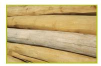
1- The different posts are made from sap free robinia. The robinia is sanded and has had its bark removed. Robinia is naturally rot proof and does not require any additional chemical protection; it is equally extremely resistant to attacks from external sources (insects, fungi, climatic variations), guaranteeing the long term durability of the playground equipment.
