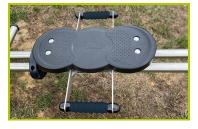
19-The Rowing machine seat is made of rubber. The handles are made of PVC.
