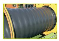
**3- The tunnel** is made of 100% recycled rotomolded polyethylene, 45cm in diameter (RAL 9005).
