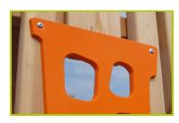
**4- The porthole** is made from lacquered Marine plywood. The colour is applied by electrostatic spraying of two-component polyurethane lacquer that is free of heavy metals, to ensure high levels of resistance to potentially aggressive chemicals such as anti-graffiti cleaning products.
