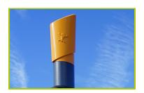
1- The 102mm diameter post is made of painted galvanised steel. The grained finish has a slightly undulating surface for increased scratch resistance. The cap is made of rotary moulded polyethylene.
