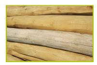
1- The posts with average diameter 120 to 140mm are made from sap free robinia. The robinia is sanded and has had its bark removed. Robinia is naturally rot proof and does not require any additional chemical protection; it is equally extremely resistant to attacks from external sources (insects, fungi, climatic variations), guaranteeing the long term durability of the playground equipment.
