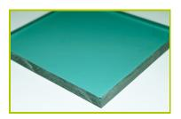
**14-The portholes** are made from 8mm thick methacrylate (PMMA).
