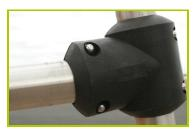
**4- Injection moulded polyamide fixings** connect the posts with the platforms and the various play features. They are non-toxic, flameproof and U.V. resistant. The thickness of the polyamide makes the equipment both strong and vandal resistant.
