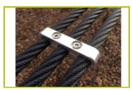
**6- The strap** is made of 3 ropes linked together with aluminium pliers. Each rope, of 16mm diameter, is made up of galvanized steel cables covered in polypropylene.
